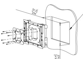
1. CUT OPENING - BOARD THICKNESS 10mm [0.39"] UP TO 21mm [0.83"] (FOR BOARDS UP TO 32mm [1.25"] THICK, REINSTALL CAM LATCHES UPSIDE DOWN.
