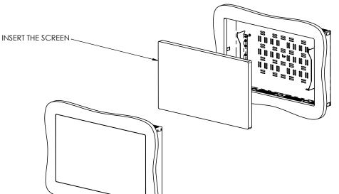
TO **INSERT** THE SCREEN INSERT THE BOTTOM EDGE OF THE SCREEN IN TO THE MOUNT AND THEN PUSH IN THE TOP.
