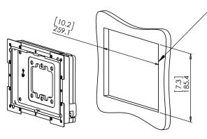
1. CUT OPENING - BOARD THICKNESS 10mm [0.39"] UP TO 21mm [0.83"] (FOR BOARDS UP TO 32mm [1.25"] THICK, REINSTALL CAM LATCHES UPSIDE DOWN.
