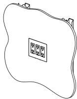
MAINTENANCE: USE TESTING SCREW DRIVER TO REMOVE TOP FACE PLATE
