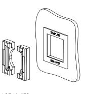
4. INSERT AND ATTACH TO THE BACK OF THE BOARD 2 BASE UNITS APPLY STRUCTURAL ADHESIVE (MS POLYMER) (ADHESIVE IS NOT PART OF THE KIT)
