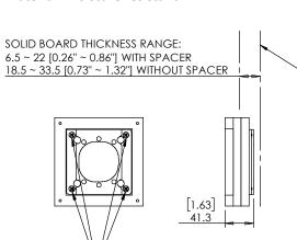
IN CASE OF INSTALLATION IN WOOD USE SCREWS, OTHERWISE APPLY STRUCTURAL ADHESIVE
