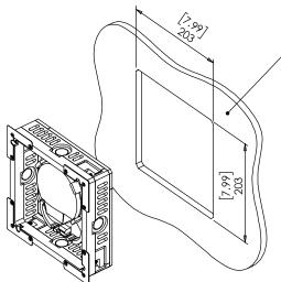
/1. CUT OPENING - Board thickness: 10mm[0.39"] up to 19mm[0.75"].
