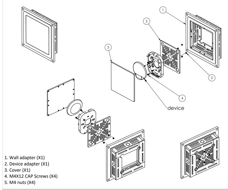
INNER SIDE WALLS ENABLE INSTALLATION OF 1/2" CONDUIT CONNECTION (NOT INCLUDED).
