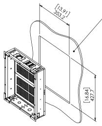
CUT OPENING - Board thickness: 10mm[0.39"] up to 19mm[0.75"].
