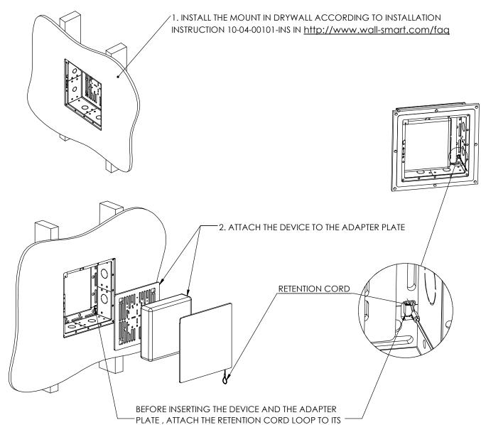
3. INSERT THE DEVICE AND THE ADAPTER PLATE INTO THE MOUNT
