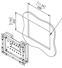
/1. CUT OPENING - BOARD THICKNESS 10mm [0.39"] UP TO 21mm [0.83"] (FOR BOARDS UP TO 32mm [1.25"] THICK, REINSTALL DOG EARS UPSIDE DOWN.
