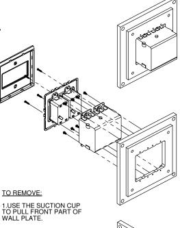
2.USE A SCREWDRIVER TO DETACH WALL PLATE
