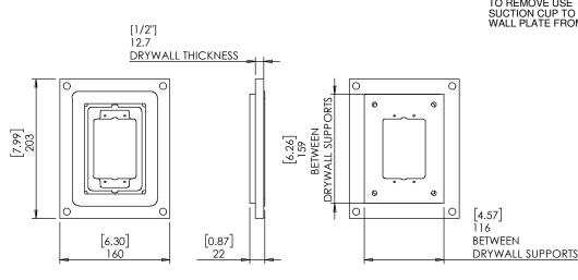
TO REMOVE USE THE SUCTION CUP TO PULL WALL PLATE FROM FRAME
