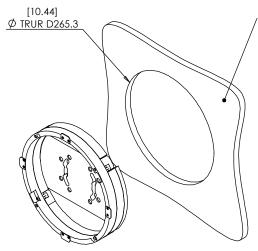
1. CUT OPENING - BOARD THICKNESS 10mm [0.39"] UP TO 22mm [0.86"] USE PAGE 3 FOR ROUTING TEMPLATE
