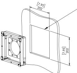
CUT OPENING - BOARD THICKNESS 10mm [0.39"] UP TO 22mm [0.86"] (FOR BOARDS UP TO 32mm [1.25"] THICK, REINSTALL CAM LATCHES UPSIDE DOWN.
