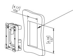
1. CUT OPENING - BOARD THICKNESS 10mm [0.39"] UP TO 21mm [0.83"] (FOR BOARDS UP TO 32mm [1.25"] THICK, REINSTALL CAM LATCHES UPSIDE DOWN.
