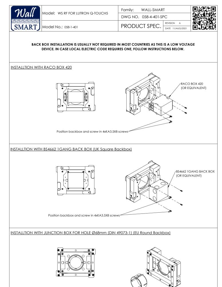
1gang junction box for hole Ø68mm Dimensions to DIN 49073-1 (Not included)
