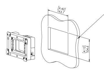
CUT OPENING - BOARD THICKNESS 10mm [0.39"] UP TO 21mm [0.83"] (FOR BOARDS UP TO 32mm [1.25"] THICK, REINSTALL CAM LATCHES UPSIDE DOWN.
