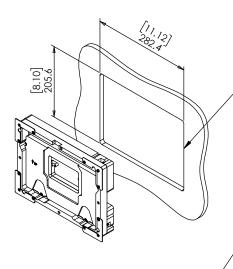
CUT OPENING - BOARD THICKNESS 10mm [0.39"] UP TO 21mm [0.83"] (FOR BOARDS UP TO 32mm [1.25"] THICK, REINSTALL CAM LATCHES UPSIDE DOWN.
