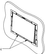
**REMOVE SCREEN:** PULL BOTTOM PART OF SCREEN AND LIFT FROM TOOTH
