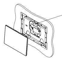
6. INSERT SCREEN: HANG SCREEN ON BACK UNIT TOOTH AND DROP IN TO PLACE
