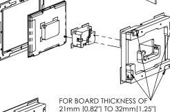
21mm [0.82"] TO 32mm[1.25"] REINSTALL CAM LATCHES **UPSIDE DOWN**
