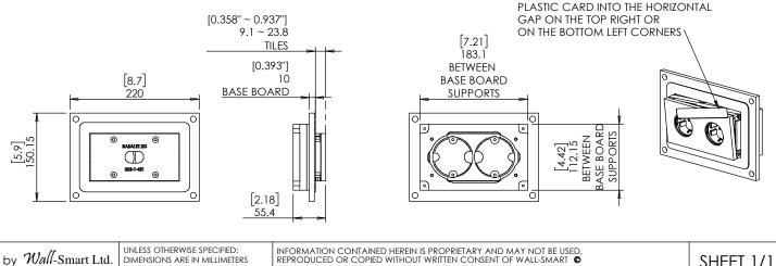
One-gang junction box for hole Ø68mm Dimensions to DIN 49073-1 (Not included)
