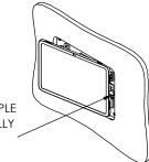
TO MOUNT THE IPAD INSETRT APPLE CONNECTOR AND MAGNETICALLY DROP iPAD IN PLACE
