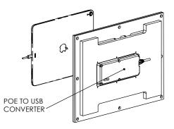
TO MOUNT THE iPad INSERT APPLE CONNECTOR AND MAGNETICALLY DROP iPad IN PLACE.
