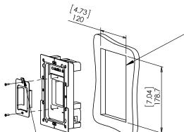
. CUT OPENING - BOARD THICKNESS 10mm [0.39"] UP TO 21mm [0.83"] (FOR BOARDS UP TO 32mm [1.25"] THICK, REINSTALL CAM LATCHES UPSIDE DOWN.
