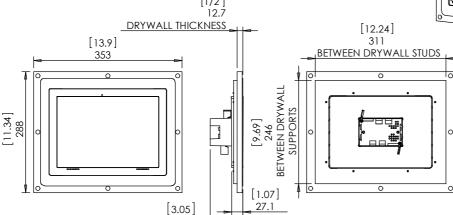
Optionally, The foam pads may be attached to the back of the 200-00420-A Install screen according Control4 manual 200-00387-D
