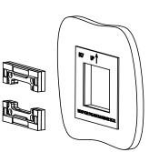
4. INSERT AND ATTACH TO THE BACK OF THE BOARD 2 BASE UNITS APPLY STRUCTURAL ADHESIVE (MS POLYMER) (ADHESIVE IS NOT PART OF THE KIT)
