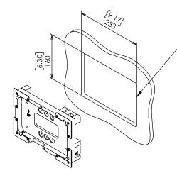
/1. CUT OPENING - BOARD THICKNESS 10mm [0.39"] UP TO 21mm [0.83"] (FOR BOARDS UP TO 32mm [1.25"] THICK, REINSTALL DOG EARS UPSIDE DOWN.
