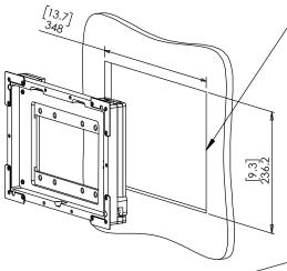
1. CUT OPENING - BOARD THICKNESS 10mm [0.39"] UP TO 18mm [0.83"] (FOR BOARDS UP TO 26mm [1.02"] THICK, REINSTALL CAM LATCHES UPSIDE DOWN.
