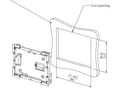
Insert wall mount and gently screw clockwise 4 retention screws until the cam latches retain the unit.
